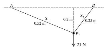
A particle P of weight 21 N is attached to one end of each of two light inextensible strings,  $S_1$  and  $S_2$ , of lengths 0.52 m and 0.25 m respectively. The other end of  $S_1$  is attached to a fixed point A, and the other end of  $S_2$  is attached to a fixed point B at the same horizontal level as A. The particle P hangs in equilibrium at a point 0.2 m below the level of AB with both strings taut (see diagram). Find the tension in  $S_1$  and the tension in  $S_2$ . [6]
